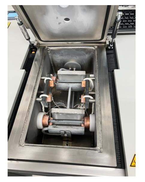
Easy access to the vacuum chamber for comfortable inserting and removing the ceramic rods
